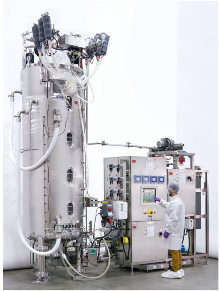
Figure 1: Single-use 1000 L fermenter holder and control unit.
