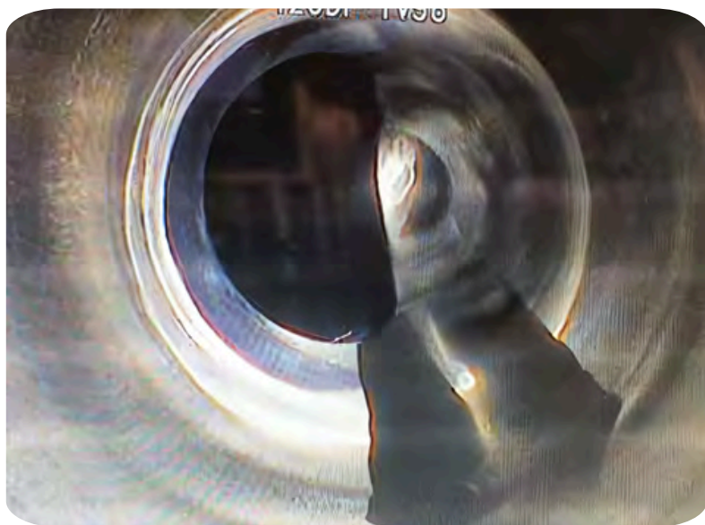
Image Details: Handling for alignment dented the filter housing, increasing contamination risk at the ferrule.
