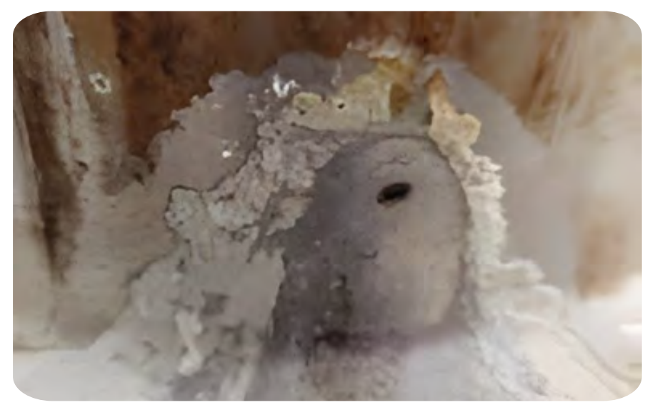
Image Details: 25,000L vessel corrosion and pitting on the top and shell seam
