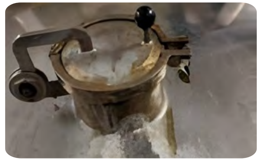
Image Details: 25,000L vessel corrosion and pitting on the top and shell seam
